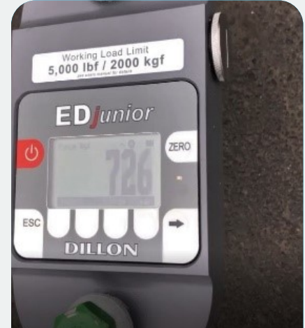
Load Cell reading at Destruction (726kgs)
